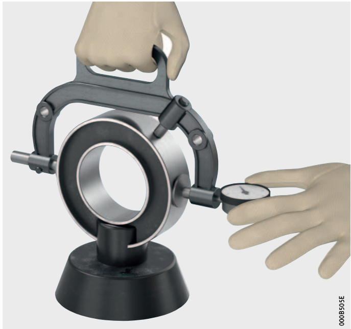
Figure 30 Setting the snap gauge using the master ring
