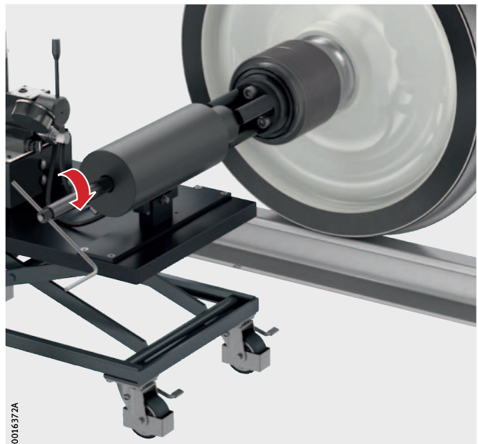
Figure 37 Screwing the spindle into the guide bush
