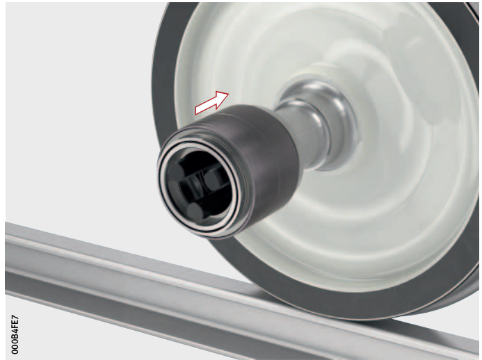
Figure 42 Sliding the TAROL unit onto the guide bush
