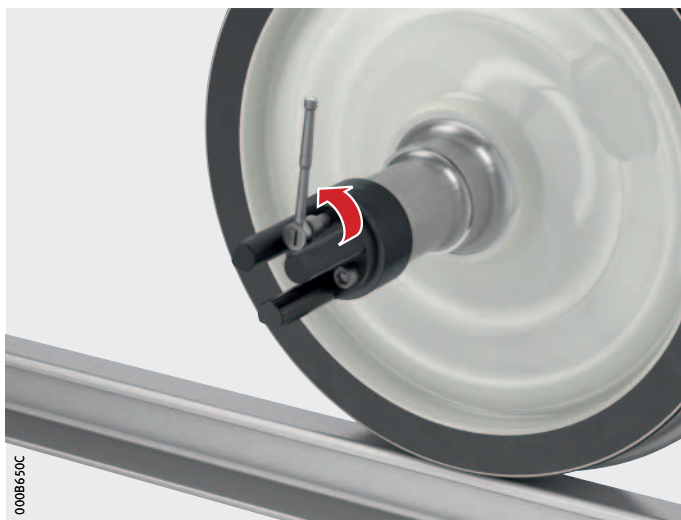
Figure 39 Unscrewing the guide bush
