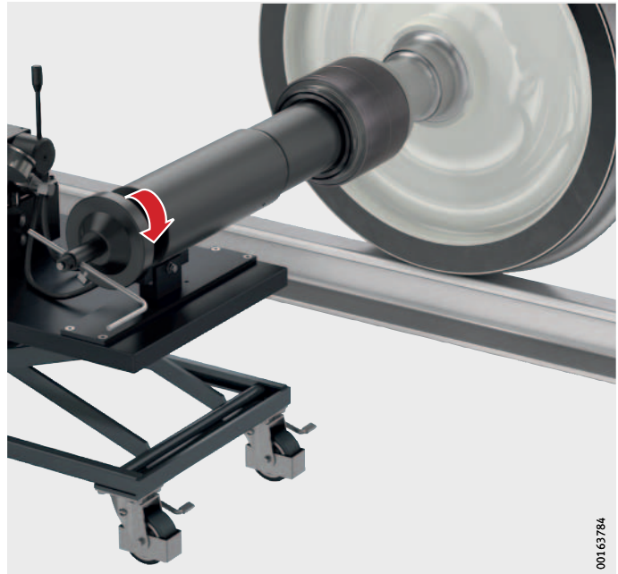
Figure 46 Screwing the spindle into the guide bush
