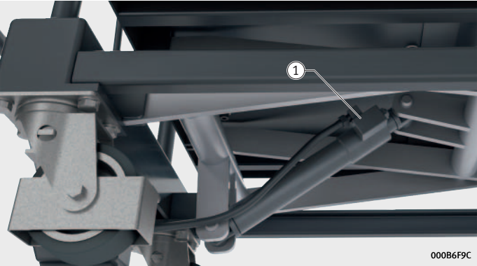
Figure 52 Bleed screw on the cylinder of the scissors lift table
