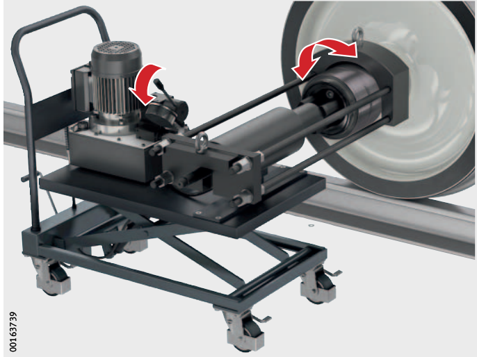
Figure 38 Extractor shoe in contact with shaft
