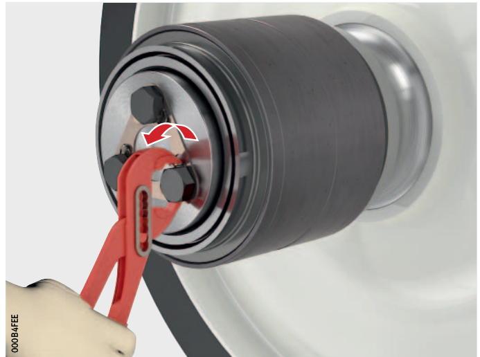
Figure 51 Bending back the tabs on the tab washer
