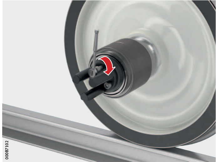
Figure 34 Screwing on the guide bush
