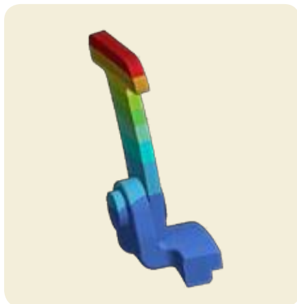
Results of a T-bar vibration analysis for a Y25 freight car axlebox
