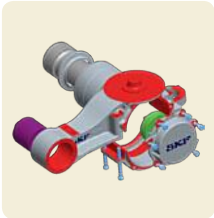
Bolts applied in an axlebox housing
