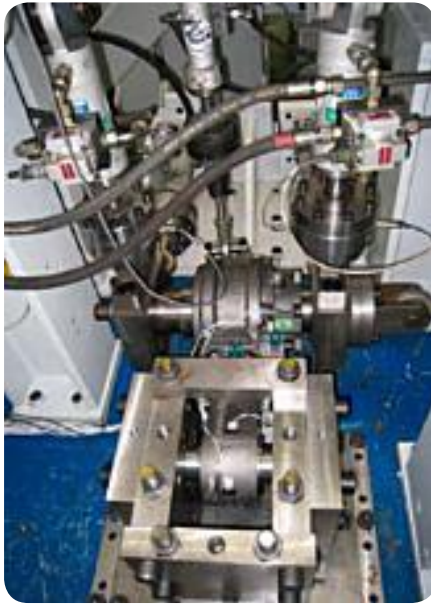
Fatigue testing of a high-speed axlebox housing
